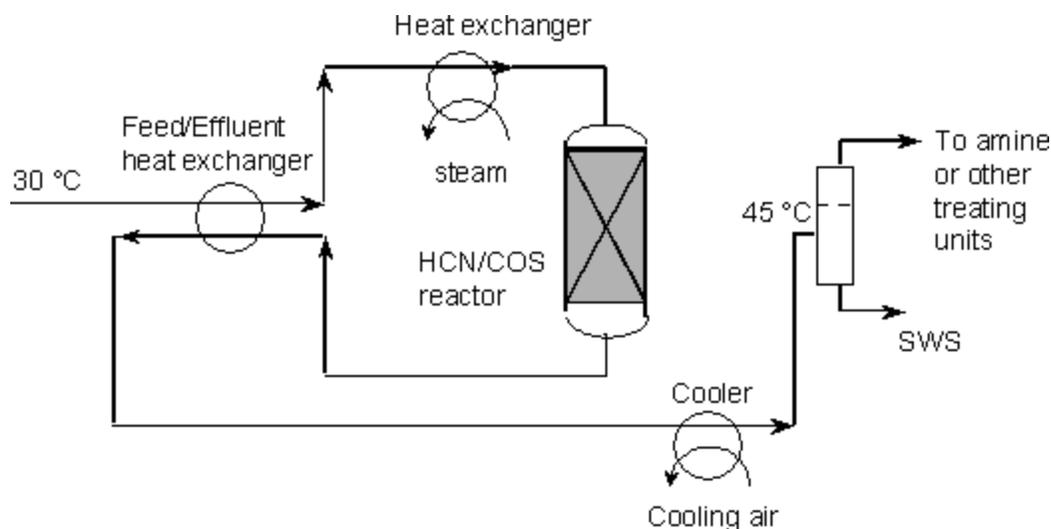
Figure 8 : The Shell HCN/COS hydrolysis process
