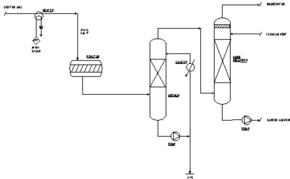
Figure 3: Shell Low Cost SCOT Process
