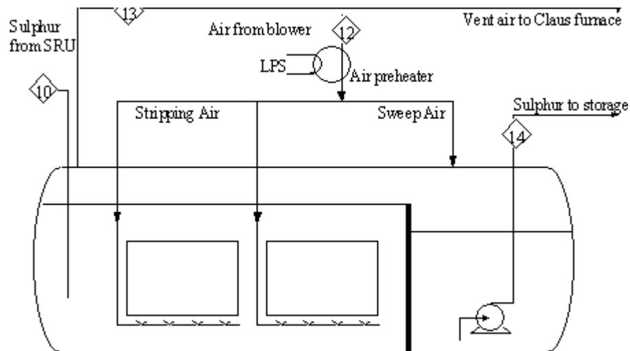
Figure 6: The Shell sulphur degassing process
