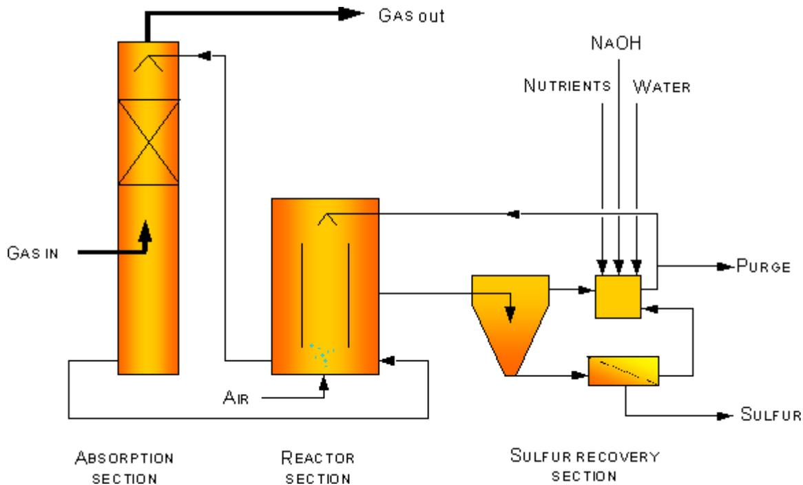
**Figure 4 : The Shell-Paques process**
