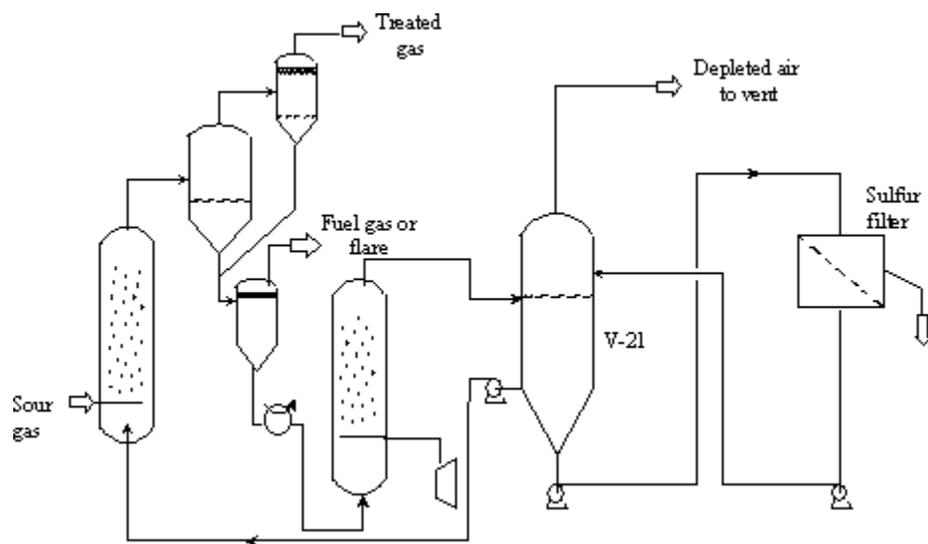
Figure 5: The SulFerox process
