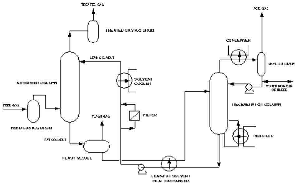
Figure 1: Typical process flow scheme of the Shell ADIP and Sulfinol Process
